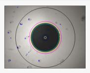
Contaminated end-face seen through the FiberCheck™ Probe Microscope
